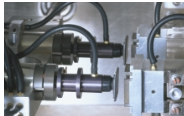
Plunge-to-board device probes transfers device to output sorter in dead-bug orientation to virtually eliminate lead damage.
